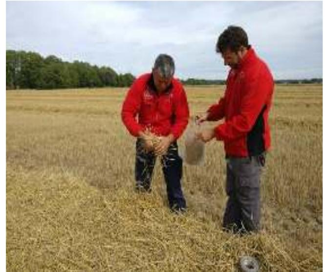
Sampling before baling to determine straw moisture content at baling
